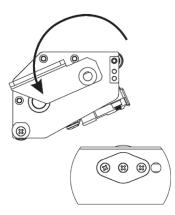
**3** Flip the Drive Roller Lift Lever clockwise to open the drive roller.
